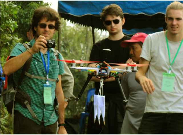
FIGURE 2. Seed bombs can be as simple as paper cones, filled with forest soil, mixed with polymer gel. The drone pictured here was made by Chiang Mai University Physics Department and releases the bombs using a simple rotating spiral (from the 1st Workshop on Automated Forest Restoration, Chiang Mai University, October 2014).
